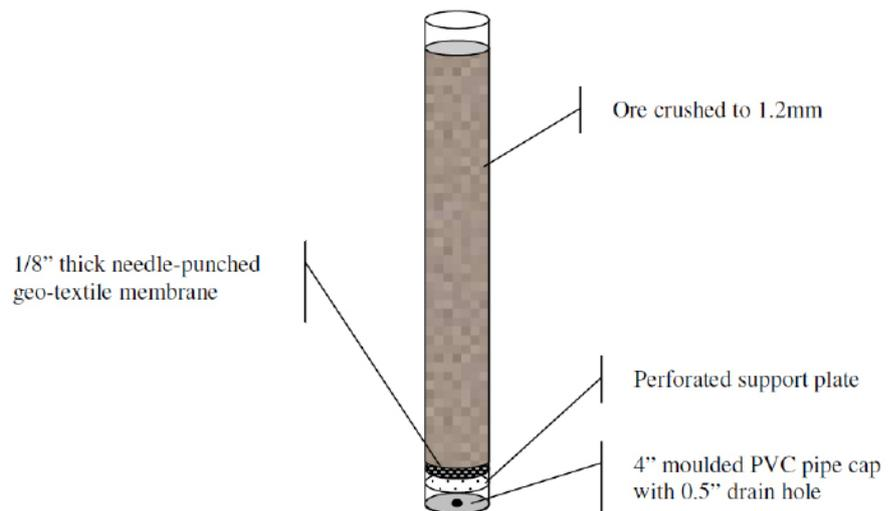
Figure 1 Ageing column schematic
