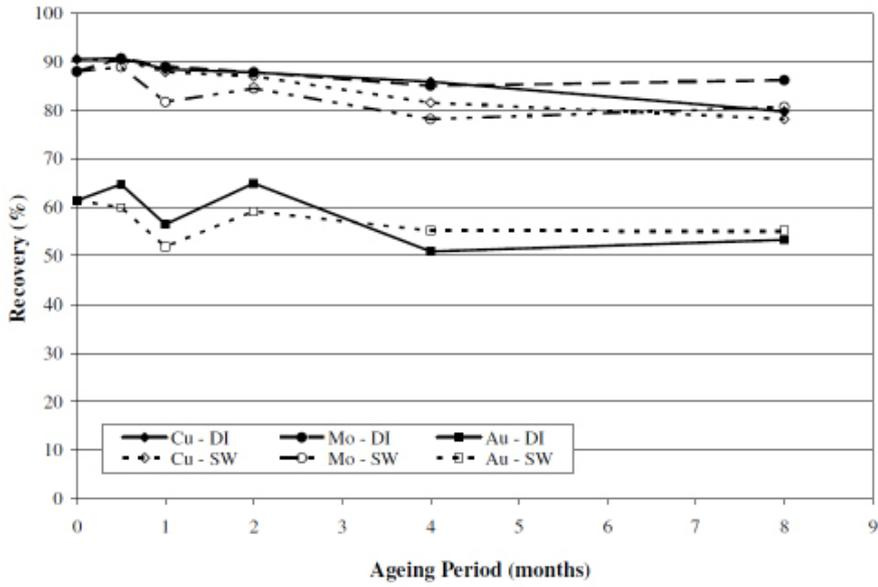
Figure 11 Cu, Au, and Mo recovery (normalized) at 26% Cu concentrate grade
