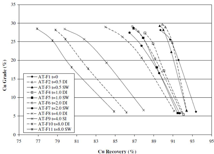
Figure 8 Cu grade-recovery curves for original AT composite and aged samples
