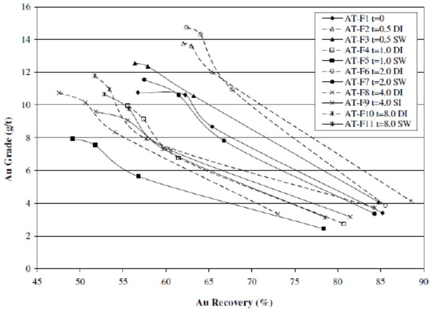
Figure 9 Au grade-recovery curves for original AT composite and aged samples
